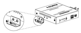
Note: Choose the wall mounting position and attach the mounting ears to the unit according to the diagram.
