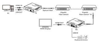
Note: It is suggested to use gigabit (1000 Mbps) switches in LAN transmission, and 100Mbps switches should not be mixed with gigabit switches when cascading.
